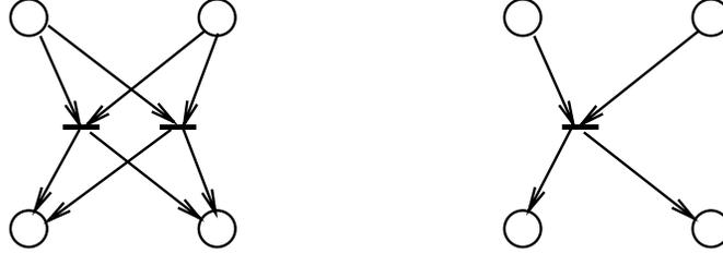
Figure 10: Example of parallel transitions reduction
